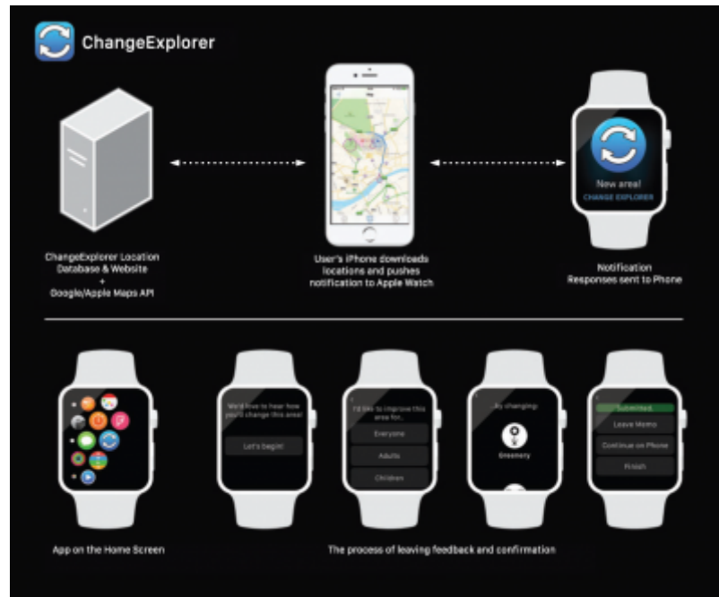
Figure 10: Operating principle of ChangeExplorer [Alexander Wilson, Mark Tewdwr-Jones, Rob Comber, 2019]
